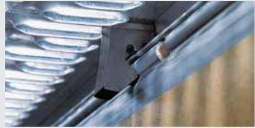
Fast locking device removes the need for bars and bolts and improves the channels hydraulic capacity. The DrainLok mechanism simply clips into the channel edge rail for quick installation. ACO's DrainLok grates are fitted with anti-shunt lugs that restrict grate movement when installed, improving durability and longevity of the system.
