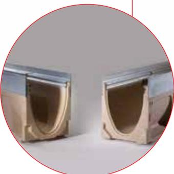
**Interconnecting end profiles** allow easy and effective joining of channels. **SF Sealant Groove** – a groove is cast into both ends of every channel. The combined groove allows for a bead of appropriate flexible sealant to be inserted at joints, if required.
