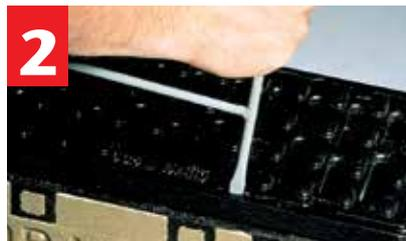
2 Rotate tool 90°; PowerLok device should push away from rail.
